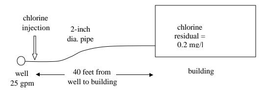
C = 0.2; Q = 25; D = 2; L = 40  $CT = 0.04 \times 2 \times 2 \times 40 \times 0.2 / 25 = 0.0512$ In this case the CT < 2.0, so this system does not provide 4-log removal.
