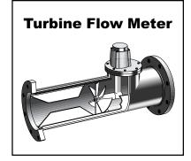
changes in the system and take corrective action before a serious problem develops. Flow meters should be equipped with totalizers to record the total amount of water pumped over a given time period.
