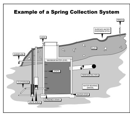
impermeable material (clay or membrane). It should be sloped away to prevent surface water from entering the collection system.
