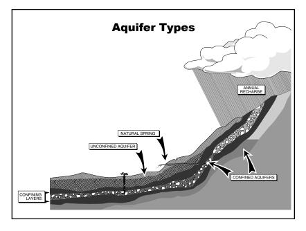
**Contamination of Unconfined Aquifers.** An unconfined aquifer rests on an aquiclude and has no confining layer above it. As a result, percolation of precipitation and infiltration of surface water from streams, lakes, and reservoirs carries water and contaminants from the surface into the aquifer. Unconfined aquifers are, therefore, considered to be comparatively vulnerable to contamination.
