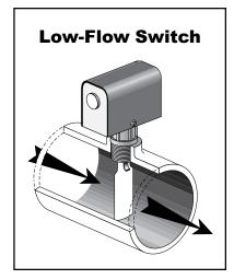
valve. This device must sense water flow or pressure in order to energize the chemical feeder. The absence of such a device has in many cases led to a significant overfeed of chemical.
