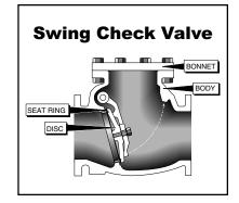
The check valve should not slam open or shut. If it does, pressure surge or water hammer conditions could be occurring in the distribution system, resulting in breaks in the mains or service lines. When the pump is not running, the drive shaft should not spin backwards. Backspin is an indicator that the check valve is not functioning and, in some cases, could lead to the impeller actually spinning off of the drive shaft.
