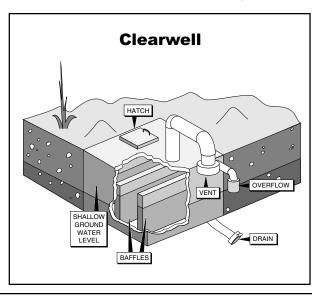
in the clearwell, often with baffling, to ensure adequate CT (CT in mg-min./L = contact time in minutes X disinfectant residual in mg/L). See Chapter 6 for a more complete explanation of CT.
