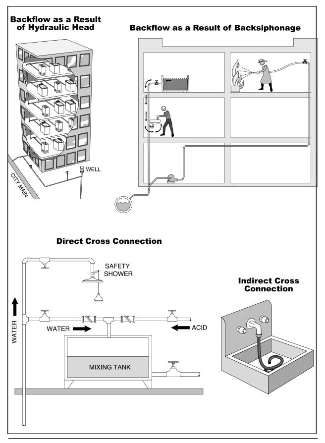
contamination of the water for the entire building (as well as threaten the water facility's supply) if the pressure of the contaminated water exceeds that of the potable water.
