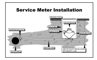
These meters are used to determine the amount of water sold. They also are used to determine unaccounted-for water and to identify leaks.
