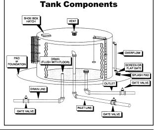
pumps fail to shut off. A screen or a closefitting flapper gate is required on the overflow to keep out birds, bugs, and mammals.
