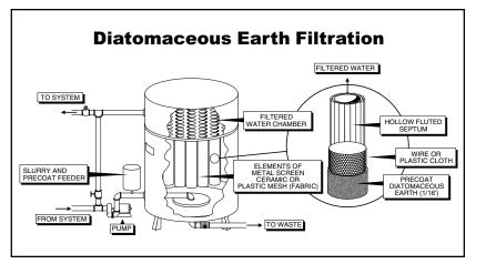
odor can be expected. The inspector should determine whether this facility has taste and odor problems that are attributable to long filter runs or prechlorination? How often is the septum inspected and cleaned (~100 filter runs)? How is the spent filter cake disposed of?
