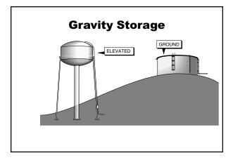
Large-Diameter Tanks Preferred. When gravity storage is used, the pressure at the head of the distribution system fluctuates with the water level in the tank. Shallow, large-diameter storage tanks are preferred over deep, small-diameter tanks because the larger diameter tanks have more water per foot of drawdown and are thus less prone to pressure fluctuations.
