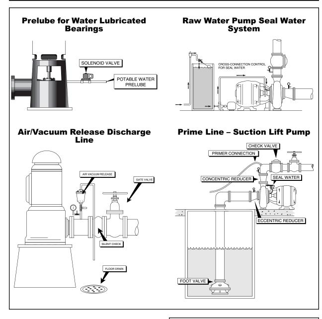
column pipe during shutdown, well pumping systems should be equipped with a foot valve (submersible well pumps) or air/vacuum relief units (vertical turbine well pumps). The inspector should determine whether the relief valve closes properly following startup and opens properly following shutdown. The discharge pipe on the relief valve should be turned downward, screened, and terminated with a suitable air-gap.
