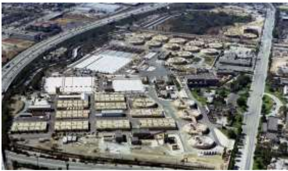
Carson, California | twenty-three 4 MG digesters
